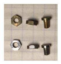
Over screws and nuts I series (brass) 1945-6— Under screws and nuts II series (nickel) post 1946
